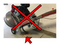
Remove the key of the dead man's switch, press the red stop button.
